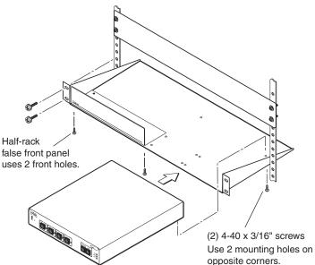
Figure 37. Mounting the IPL T PCS4 on a Rack Shelf
